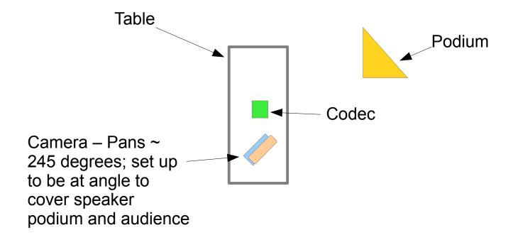
Signal Cabling – LAN to Codec; HDMI out from Codec to UCP HDMI projector input jack; HDMI from camera to HDMI-1 in of Codec; Audio out from Rolls MP222 preamp out (dual 1/4" maleTS to 3.5mm Line in of Codec.
